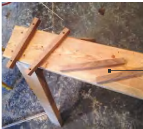
STEP 14. The support brackets for the shelves can then be cut and screwed to the sides and middle
